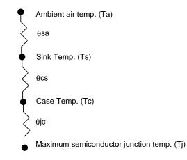
In most applications, values for all these parameters are known, and can be used as the selection criteria for the heat sink (i.e. to find a heat sink, with corresponding air flow, that provides an acceptable  $\theta$ sa). The follow equation can be used to calculate the required  $\theta$ sa, and is applicable for both natural and forced convection cooling.
