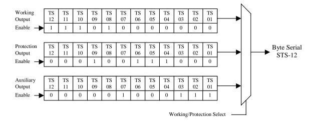
The S/UNI-MACH48 has the same capability as the TBS with the exception that it has eight byte-serial STS-12 links as opposed to twelve. The blocks are named Input Working Timeslot Interchange (IWTI) and Input Protection Timeslot Interchange (IPTI) in the ingress direction toward the system side of the S/UNI-MACH48 and Output Working Timeslot Interchange (OWTI) and Output Protection Timeslot Interchange (OPTI) in the opposite direction.
